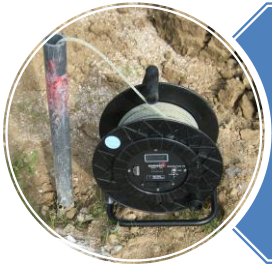
Water level indicators & other geotechnical measuring devices
